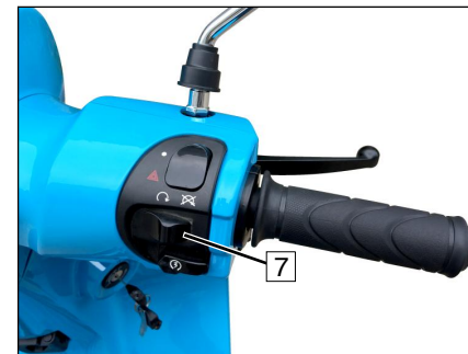
5. Right switch(7) at "↻" position.
