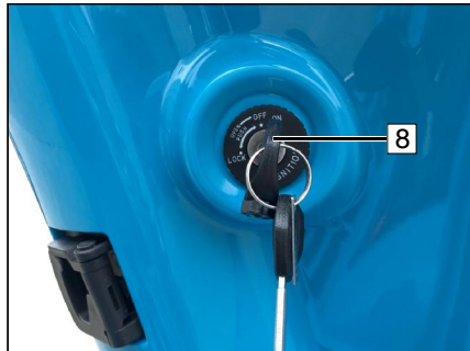
6. The ignition key(8) at "↻" position.
