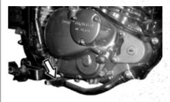
Press down this pedal to apply rear wheel brake, and the brake indicator light is lit.
