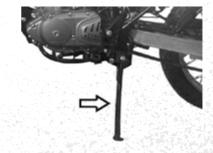
The vehicle is provided with a side stand on the left side.
