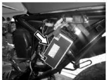
The fuse box is located inside the guard board on the right side of the chassis. A fuse is provided for all the electrical system. In case of any trouble to electrical system, check the fuse first. If the fuse is blown out, replace it with the spare fuse (15A) in the fuse box.
