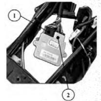
Press ECU towards plug-in direction gently. After a "snap" sound, it is installed into position.
