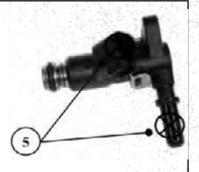
A: align fuel injector with corresponding position of air inlet elbow; screw it in installation hole slowly, with axial pressing force less than 500N as shown in 4.
