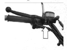
The switch of front brake light is located below the brake grip. Loosen the screw and move the switch position back and forth to find a proper point so that the lamp is lit immediately when pressure is applied but before the grip is fully pressed.
