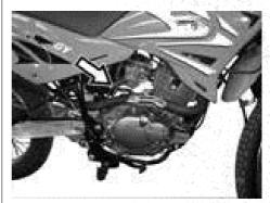
The kickback start lever is installed on the right side of the motor. Owing to motorial kickback starting mechanism, the engine can be started in any gear position provided the clutch is released.
