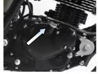
3. Remo g from strainer cover on the engine bottom to drain oil.
