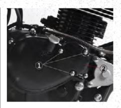
5. Remove filter element cover, pull out oil filter element and replace it with a new one.
