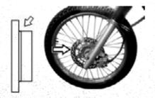
The essential of checking the front wheel brake lining is to see if the lining is worn to the limit mark. If wearing exceeds the mark, the brake lining shall be replaced with a new one.
