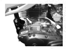
Chassis number (or VIN code) and engine number is necessary for registration of your motorcycle. Such numbers are needed with order components or service, to allow the distributor to provide you with better service.
