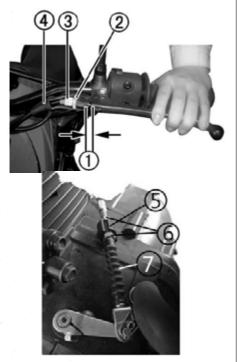
Loosen nut (2) and rotate the grip tensioning ring (3) clockwise to the stop. Loosen the wire rope adjusting ring lock nut (6), and rotate the wire tensioning ring (5) back and forth, until the grip clearance is about 4 mm. Grip tensioning ring (3) can be used for fine tuning. After the adjustment is completed, tighten locking nut (2) and (6), and cover them with
