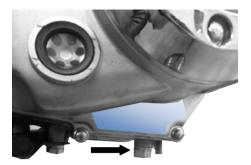
4. Tighten the oil drain ring and fill fresh engine oil into the oil filler, before gently tightening the top cover.
