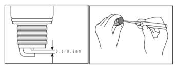
After the first 1000 km and every 3000 km thereafter, clean off any carbon deposit from spark plug by using a small steel wire brush or a spark plug cleaner. Readjust the spark plug gap with a thickness feeler to keep it between 0.6 - 0.8 mm. Replace spark plug every 6000 km.
