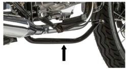
Press down this pedal to apply rear wheel brake, and the brake indicator light is lit.
